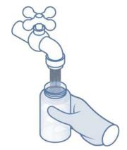
**Fill the sample bottle** to the shoulder or the line marked "250 ml" leaving a little bit of room at the top of the bottle. Close the cap tightly.
