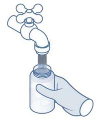
**After 30 seconds**, while the water is flowing place the sample bottle under the fixture and fill the sample bottle to the shoulder or the line marked "250 mL". Close the cap tightly.
